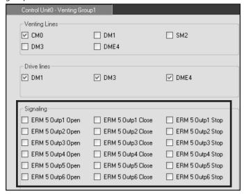
Here, the statuses of the ventilation can be assigned to the relays. "Open", "Close" and "Stop" are available for each relay. If parameters are set for a relay to display Open or Close, then Open or Close is active until there is either a change in direction of movement or a "Stop" signal is issued. The stop signal is only pending when the system is stopped manually, i.e.
