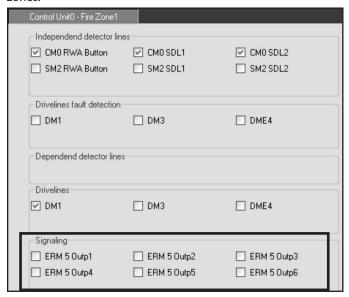
Here, selection can be made of the relays which are to be switched when an alarm occurs for this smoke zone. A relay can also be assigned to different smoke zones.
