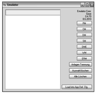
The emulator is used to simulate system set-up when the PC is no longer connected to an MBZ 300 control unit. To simulate the system set-up, the various modules are added to a list in descending order. The modules can be moved in the list by drag-and-drop. Then the system set-up is loaded to the configuration program, where the settings can be made.
