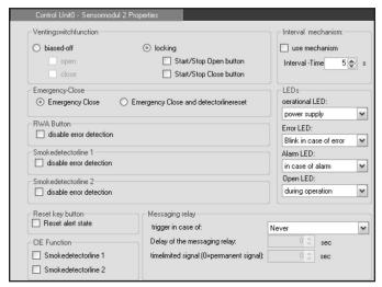
In the standard configuration the SM forms a new smoke zone. All the following DMs (up to the next SM) are assigned to this smoke zone.
